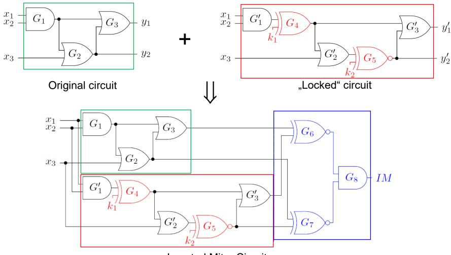
Inverted Miter Circuit
